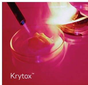
Hydrocarbon-based lubricants burn; Krytox™ does not.
